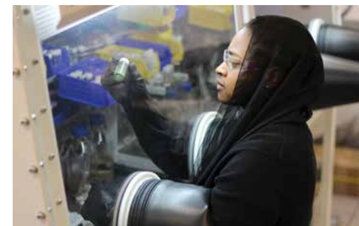
Safiyah Muhammad, a student in Alison Fout's laboratory, synthesizes new compounds in a laboratory glovebox which maintains an atmosphere free of oxygen and water. (Photo by Lauren Hagler.)
